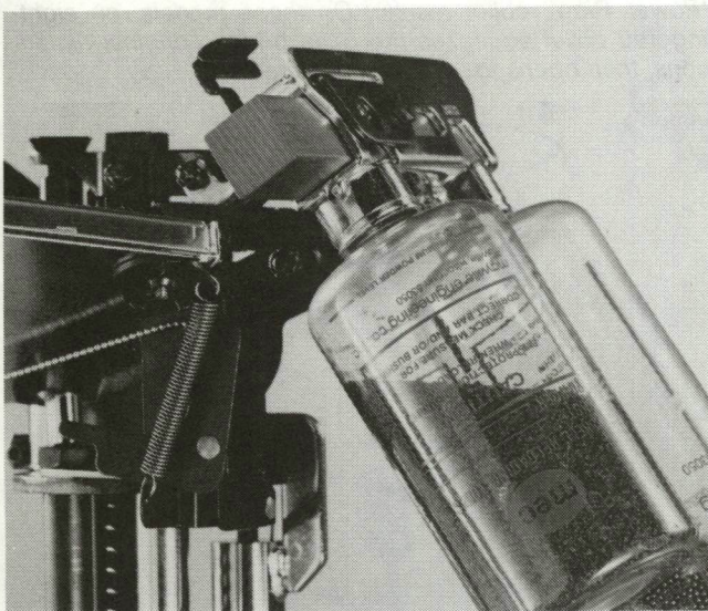
Flip-top measure permits the measuring assembly to be flipped so that the powder and shot containers are inserted and removed in the upright position to avoid spilling.
