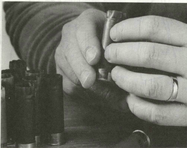
Inspect hulls for damage or foreign objects such as feathers, leaves, twigs, etc., on inside.
