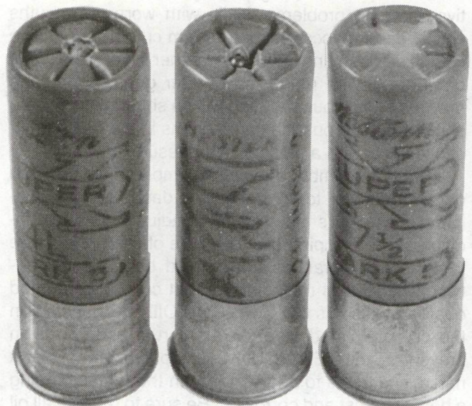
Factory Shell With Heat Sealed Crimp, Reloaded Shell Showing "Hole" and Shell with "Hole" Closed With Candle Wax.
