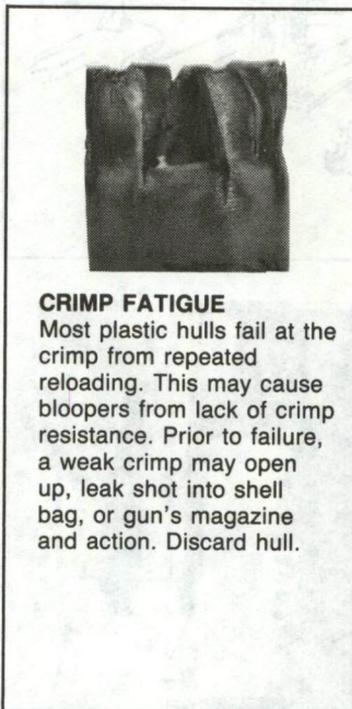
Inspect hulls for damage or foreign objects such as feathers, leaves, twigs, etc., on inside.
