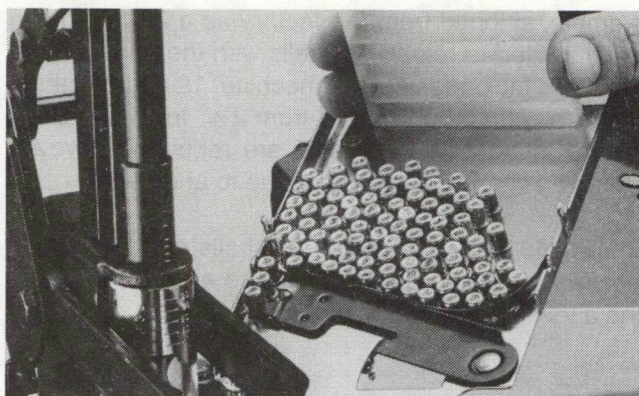
Automatic primer feed eliminates handling of individual primers. It is standard on some MEC models; an optional accessory on others.
